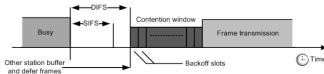
Fig 2: Timing chart for data transmission.
