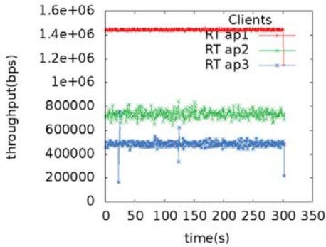
Fig. 7. Throughputs for real-time applications for single client.
