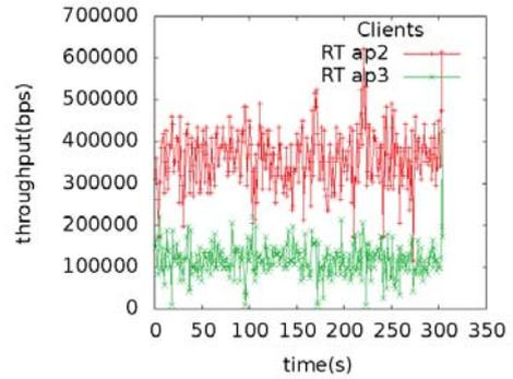
Fig. 9. Throughputs for real-time applications for two clients in line topology.
