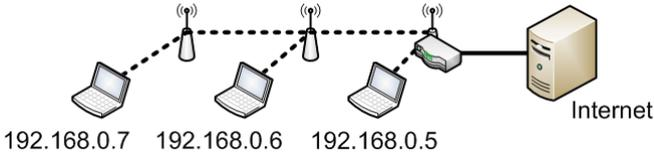
Fig. 3. Example topology for consumed bandwidth estimation.
