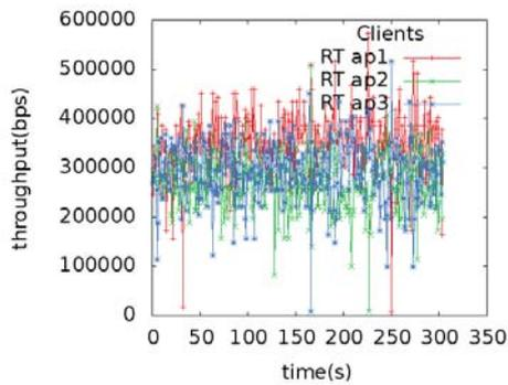
Fig. 10. Throughputs for real-time applications for three clients in tree topology.
