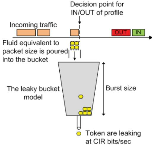
Fig. 4. Leaky bucket operation.
