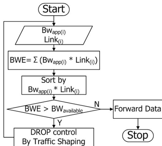
Fig. 2. Flowchart of traffic control method.
