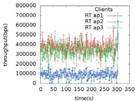
Fig. 11. Throughputs for real-time applications for three clients in line topology.
