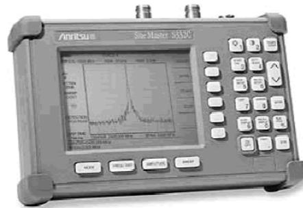
**Gambar 9.12.** Spectrum Analyzer
