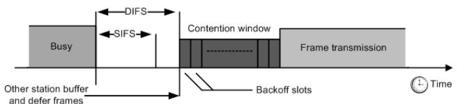
Fig. 2: Timing chart for data frame transmission.
